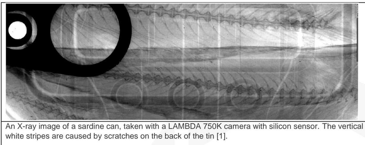
This example was one of the first demonstrations of the capability of the camera. It shows the high spatial resolution and sensitivity of the system. There are no gaps in the image; all photons that are interacting in the sensor are counted.
