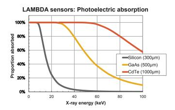
The LAMBDA 350k pixel detector is available for hard X-ray detection with GaAs or CdTe sensor layers. This provides high quantum efficiency at high X-ray energies (75% at 40keV for GaAs, and 75% at 80keV for CdTe), while retaining all other specifications of the 750k system with silicon sensor.
