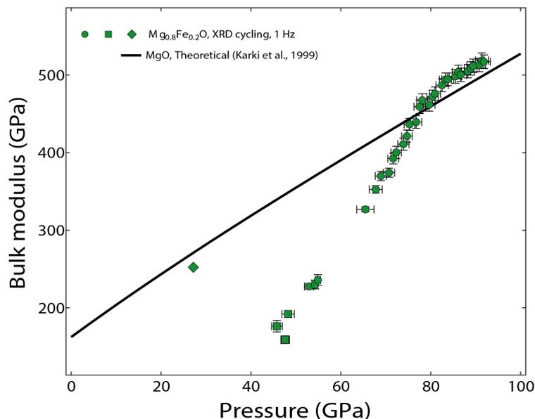
↑ Variation of the bulk modulus with pressure; the line represents the theoretical response of magnesium oxide to pressure increase. The markers refer to measurements obtained on ferropericlaste with X-ray imaging, using the setup at the Extreme Conditions Beamline at PETRA III in the presented study. © H. Marquardt, with kind approval.
