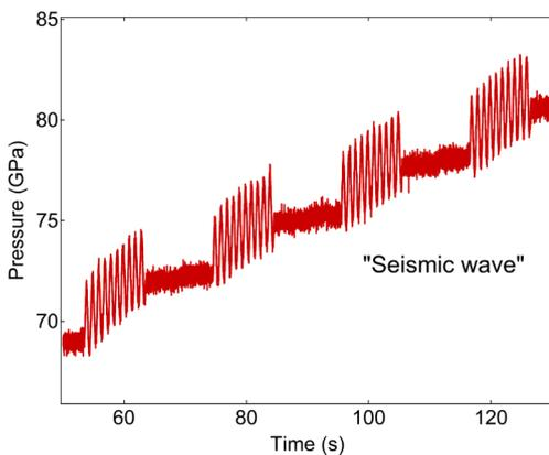
↑ Pressure oscillations realized with the dynamic Diamond Anvil Cell as simulation of a seismic wave (© H.-P. Liermann, with kind approval)
