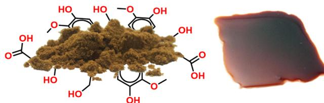
↑ Chemical structure and physical appearance of lignin (left) and a thermoset (right) that can be made from it.
