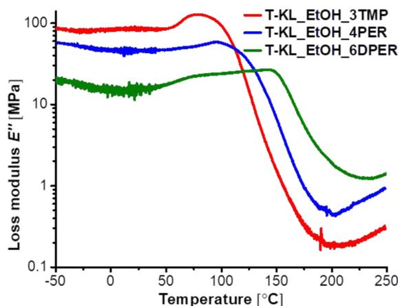
▲ Loss modulus, a property describing the elastic properties of a polymer, of the three different thermosets upon heating (“thermal curing”).
