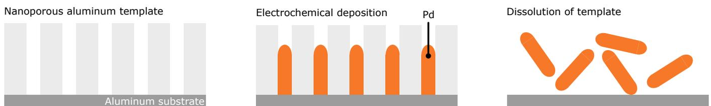
▲ Production of nanowires in a nanoporous template.
