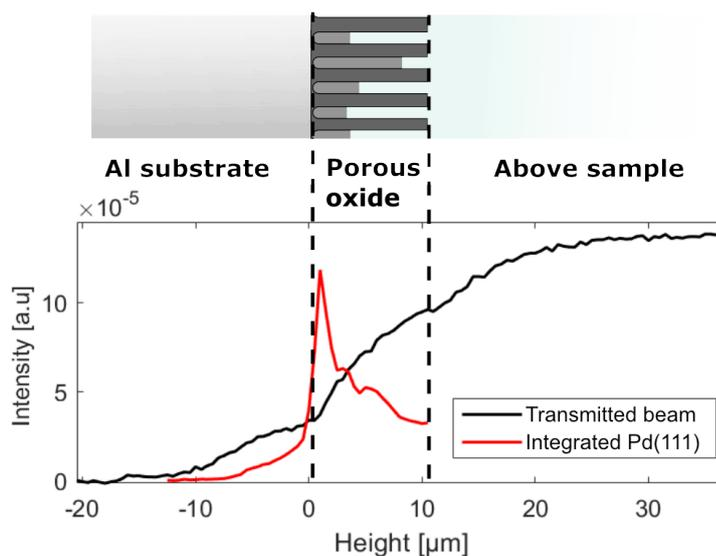
▲ Intensity of the transmitted beam signal and the integrated Pd peak after 40 minutes of growth.
