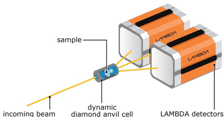
Setup with two LAMBDA 2M cameras recording diffraction images from the sample in a diamond anvil cell.
