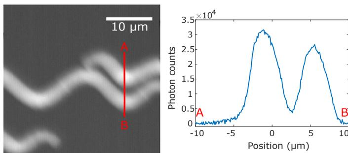
▲ Left: Spirulina SCXM image at 60 keV with 100 nm steps and 100 ms dwell time. Right: Photon counts along the red line. Adapted with permission from Villanueva-Perez et al. (2021) © The Optical Society.
