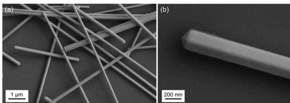
◀ Scanning electron microscopy images of (a) a silver nanowire network and (b) a single silver nanowire.
