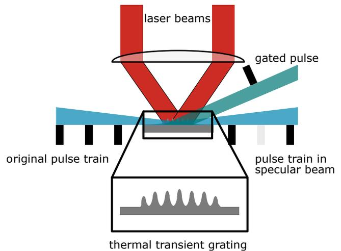
↑ Principle of thermal transient grating. The red beams represent the crossed laser beams used for optical excitation.
